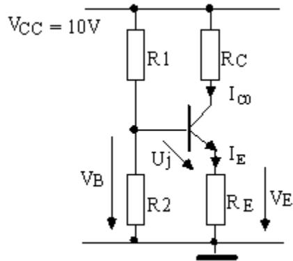
$$V_B = \frac{R_2}{R_1 + R_2} V_{CC} = 2,48 \text{ V} \quad V_E = V_B - U_j = 1,78 \text{ V}$$
