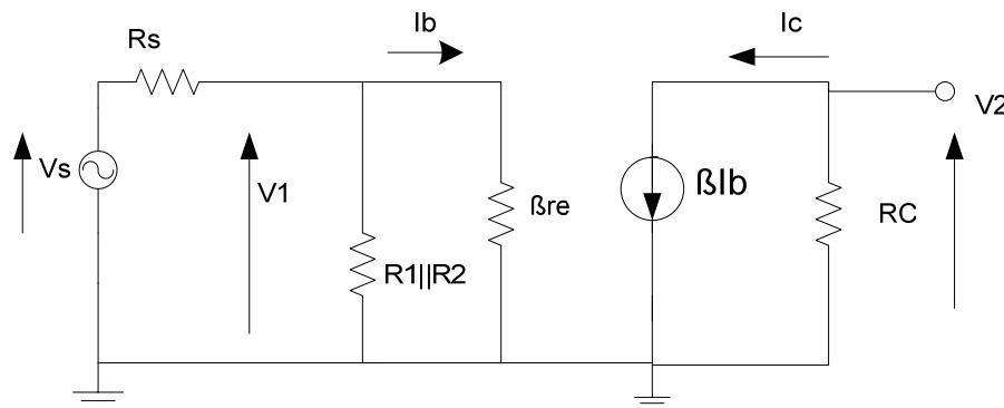
$$d) R_{in} = \frac{v_1}{i_1} = \left( \frac{1}{R_1} + \frac{1}{R_2} + \frac{1}{\beta * r_e} \right)^{-1} = 4,16 \text{ k}\Omega$$
